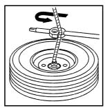
Use the wheel wrench hook that allows you to pull the hoist cable towards you, to assist in reaching the spare tire.
